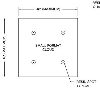
RESIN SPOT PLACEMENT & QUANTITY DEPENDENT ON CLOUD SIZE.
