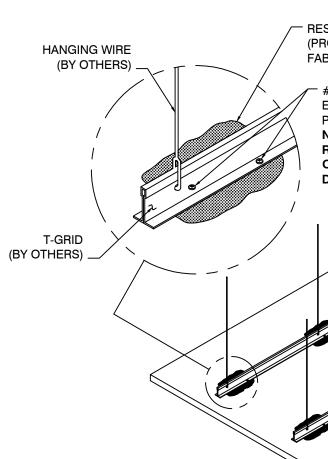
RESIN SPOT (PROVIDED BY PANEL FABRICATOR)
