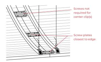
When installed, joining plates on the outside edges (usually the outside 2) are screwed to the next panel whereas this is not required for the center clips as shown.
