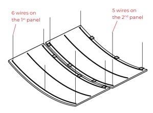
IMPORTANT – Note offset installation of Joining Clips (6 per 8' length as shown). Also Note: Factor of Safety on the "Following Panel" above is 8.0!
