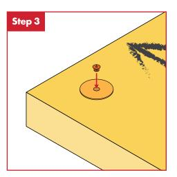
Insert reusable marking plugs into the Snap-On anchors. Chalking the of the marker may help see the mark.
