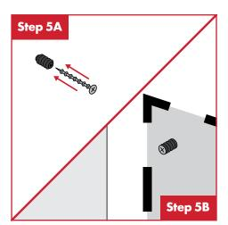
Screw ratchets to surface at marked locations. Flat end of ratchet goes against the surface, curved end faces out. #8 screws recommended.\*
