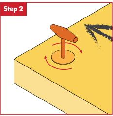
Screw Rotofast Snap-On Anchors into back of the panel using the Rotofast driver tool. For one inch panels, only insert the driver tool halfway into the anchor.\* \*Do not overtighten.
