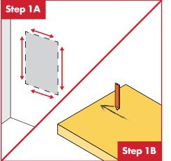
Measure and mark the location where panel will be placed and mark the orientation on the back of the panel.
