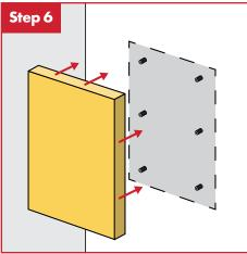
Firmly strike panel onto ratchets to complete the installation.
